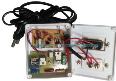
Fig.7: Home Automation using IOT Project Circuit
