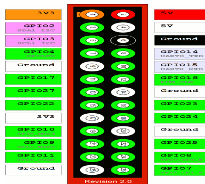
Fig.4: GPIO pin configuration
